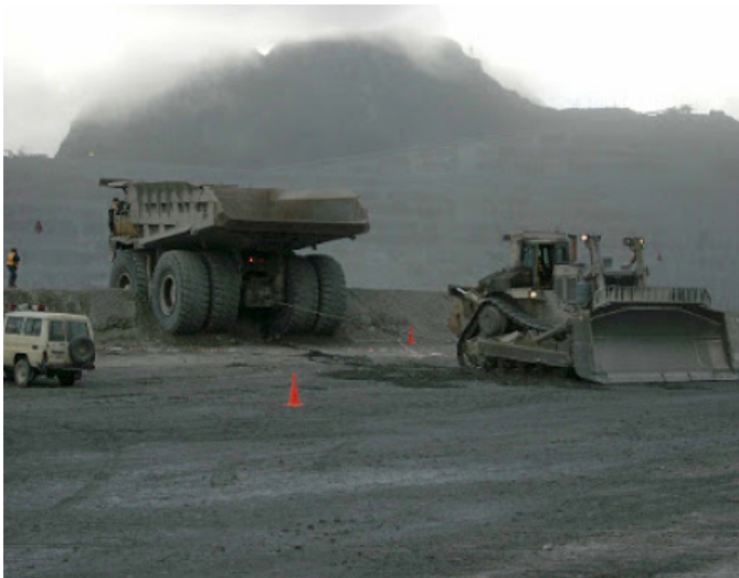
Truck damage from poor ramp designs causing stress on steering frame and axles
