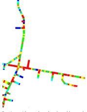
Section with overbreak colored by each cut. At present, design stripping is not taken into account.
